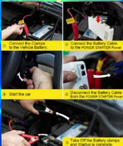
Vehicle Jump Start - How to use It for Jump start
